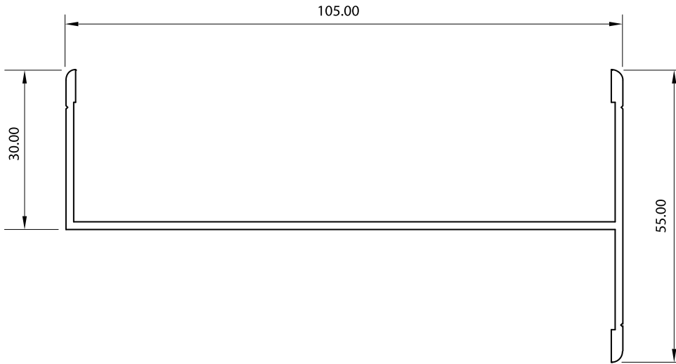
Section No. F3585 100mm Chair Section 0.777kg/m, per 377
