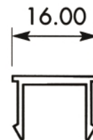
* Section No. 5706 Pocket infill 0.122 kg/m, per 75
